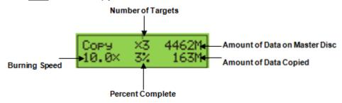
3. Once the copy task is finished, the copied discs will be ejected and the result of copy task will show on the LCD:
