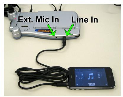
portable audio device. Use a 1/8" Stereo Mini Plug to Mini Plug cable (Sold Separately) and plug your device in. Adjust the volume on your device to ¾ of its maximum and adjust the Line Volume and Master Volume controls on the SL935 to suit.
