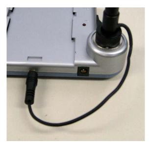
4. Connect the included speaker wires to the left and right speakers. Bare leads attach to the speaker end, 1/8" mini plugs go to the amplifier.
