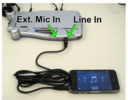
audio device. Use a 1/8" Stereo Mini Plug to Mini Plug cable (Sold Separately) and plug your device in. Adjust the volume on your device to ¾ of its maximum and adjust the Line Volume and Master Volume controls on the SL930 to suit.
