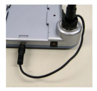
4. Connect the speaker wire from the flat panel speaker to either the left or right speaker output.
