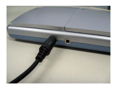
5. Insert power plug in to jack below microphone mount
