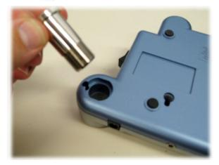
through the bottom. It will push out a blanking plug and pop-out the top of the amp.
